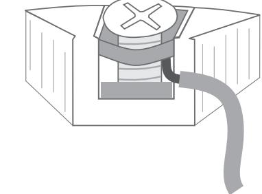
Wires must be mounted between the metal plates.
